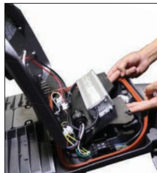
Safety switch to cut off power supply once cover opened
